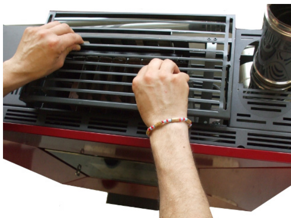
Fig. 53 - Remove upper grid
