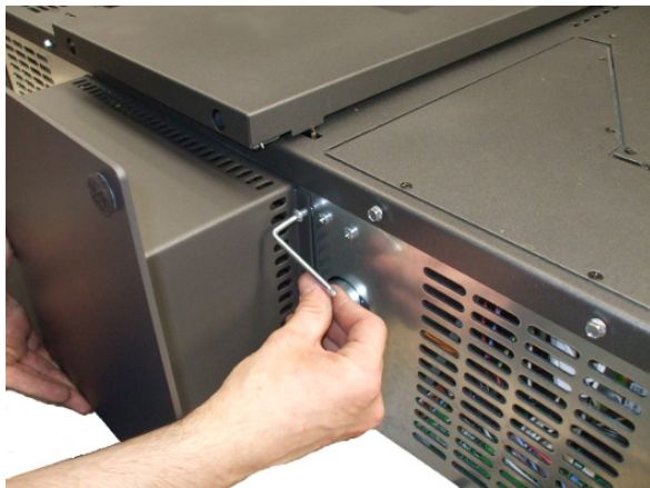
Fig. 15 - Assembling the pedestal
