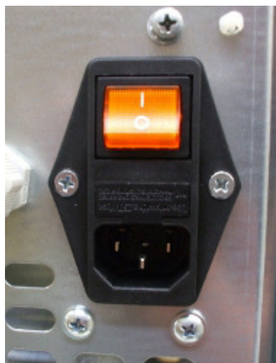
Fig. 33 - Electric socket with master switch
